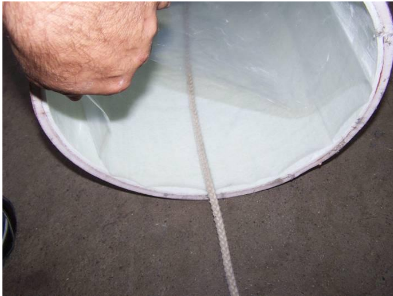
Figure 10: Release of inner film after curing
